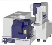
Rigaku DSC Vesta DSC quantifies the energy changes in reaction such as melting, crystallization and etc.
